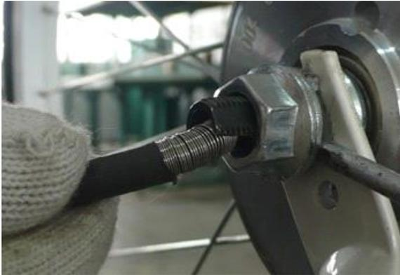
**IMPORTANT:** *Make sure that the torque washer fits firmly inside the fork/rear drop-outs and is completely stable. If the torque washer doesn't fit properly, contact a local bike service shop for assistance on finding a different washer or replacing the fork altogether. Remember that damage caused by motor "spin outs" is not covered by the warranty.*
